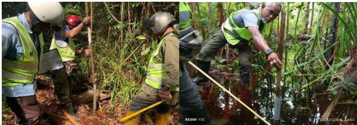
Figure 9. Piezometer reading done by the community patroller
